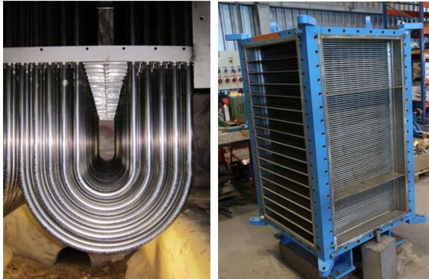
Figure 13: Applications of alloy UNS N06058 for example as a heat recovery system in a FGD plant (left) or as a heat exchanger in the chemical process industry (right).
